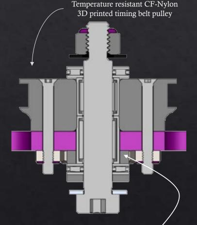
Needle-roller bearings distribute impact forces along shoulder bolt
