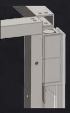
Frames assemble by being stacked at peg & tube joint at vertical bracket
